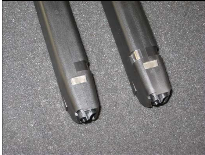
Gen 4 mag (right) has extra notch on side
