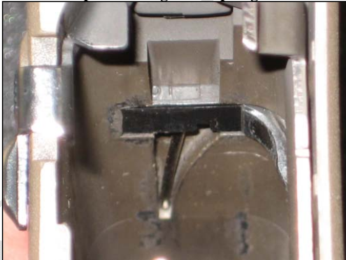
v shaped G4 mag catch spring notch
