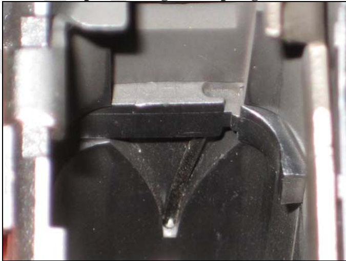
v shaped G4 mag catch spring notch
