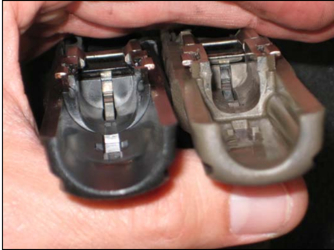
r shaped G3 mag catch spring notch
